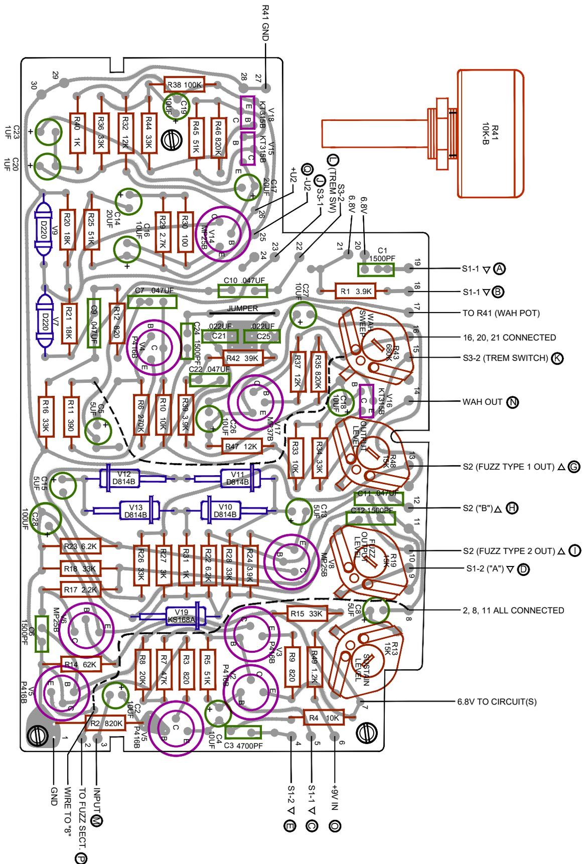
**NOTE:** On some examples V19 and R49 are not present; R49 is replaced by a jumper. There is no provision whatsoever for V19 - no holes were provided in the PCB.
